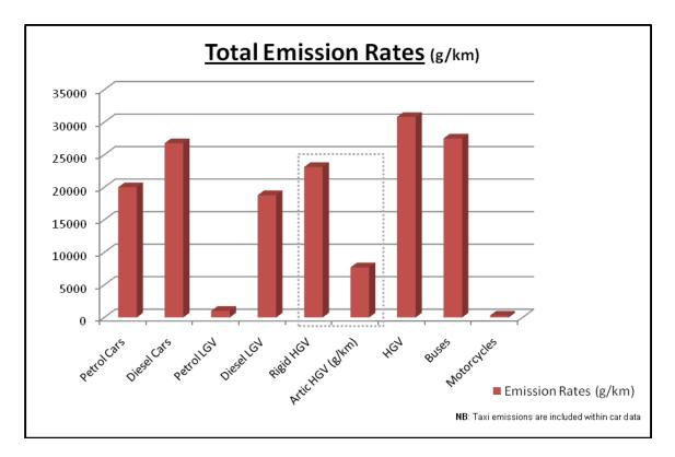
Figure 4.2 Total NOx Emission Rates by Vehicle Type (sum of all road links)
