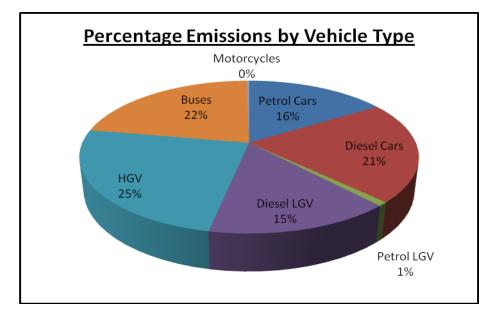
Figure 4.3 Percentage NOx Emissions by Vehicle Type (sum of all road links)
